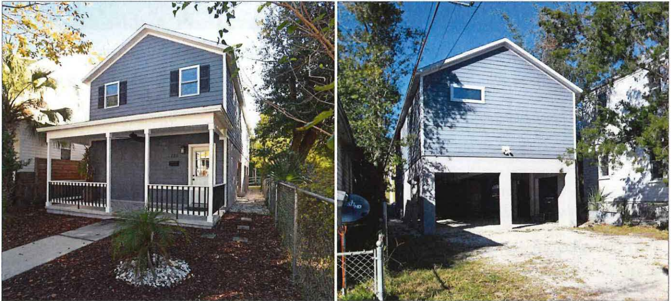
In this example of wet floodproofing of a new residence in Lincolnville, the front elevation (at left) is compatible with scale, form, and stylistic components of many of the neighboring houses. The ground level parking area is accessed from the rear and could be largely concealed with vegetation.
