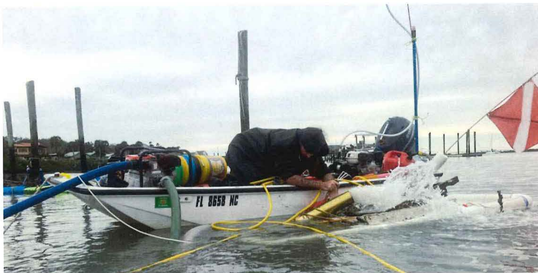
Figure 27. The 13' Boston Whaler Indy anchored near excavation Unit 1, in the deeper water outside the oyster bar. The water pump is mounted at the bow, and the screendeck is tied off on the port side (foreground). The dredge head is spewing water and spoil into the screen from the divers' excavation below. 22 December 2022 photograph by Chuck Meide.
