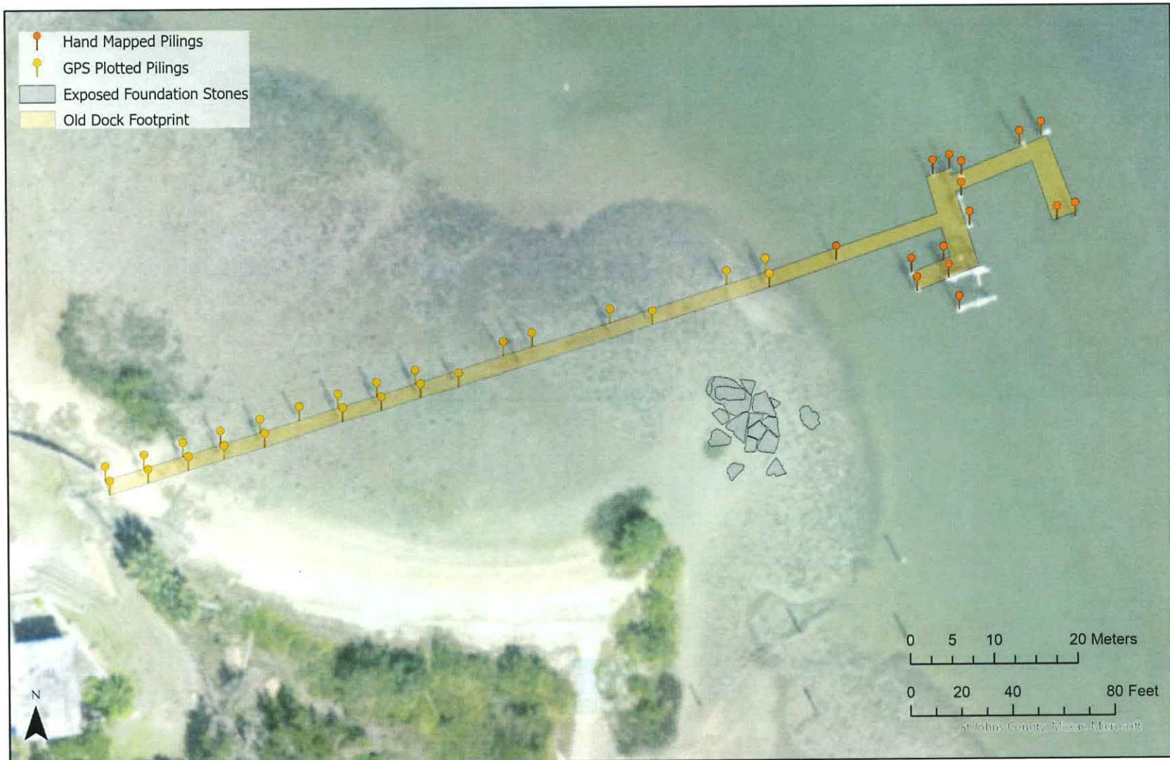
Figure 39. Location of the exposed foundation stones in relation to the footprint of the old dock. Existing dock pilings are plotted using sub-centimeter accurate GPS for those accessible on the foreshore, and traditional mapping with measuring tapes for those in the water at low tide. Image by Airielle Cathers.
