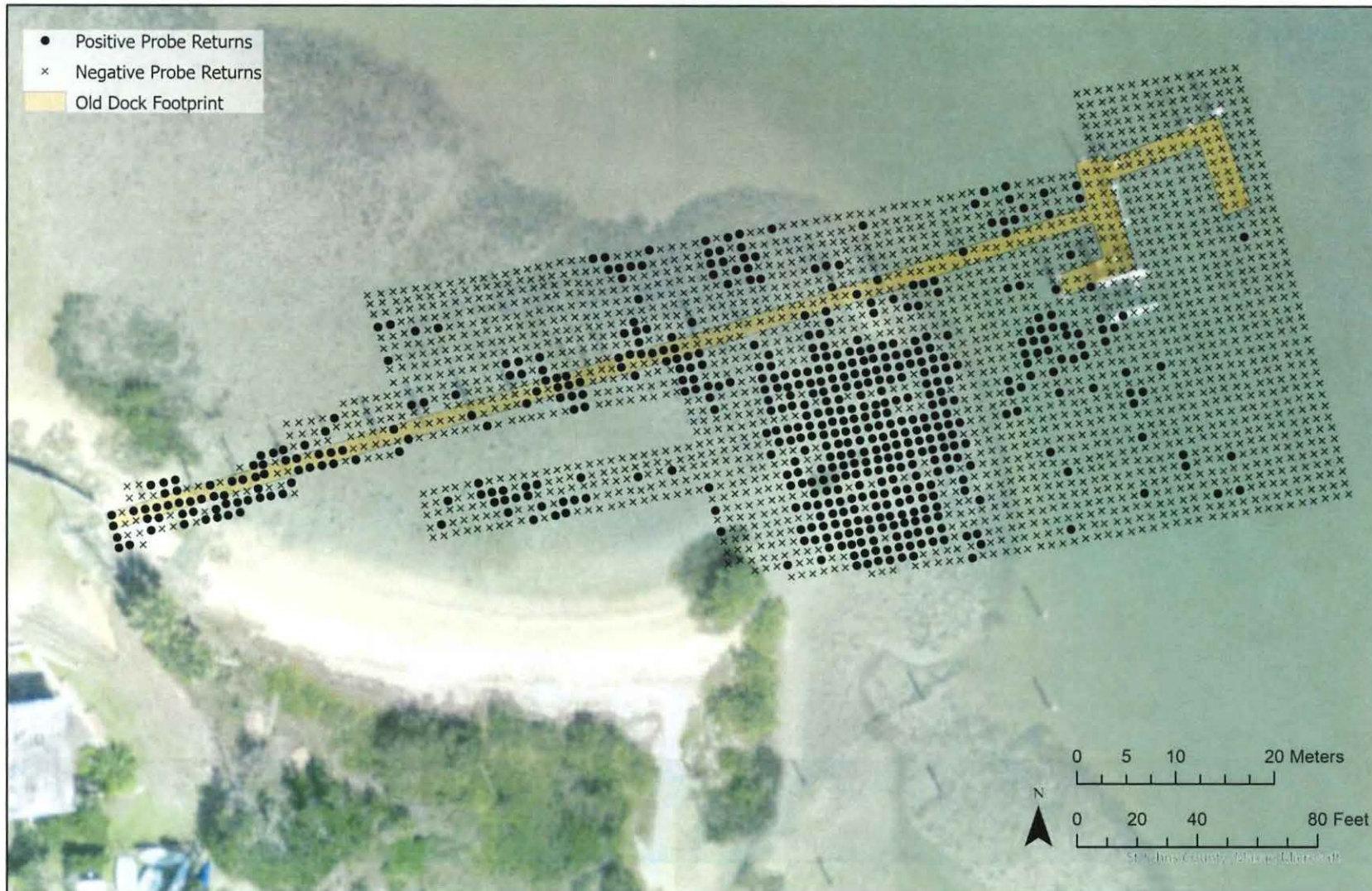
Figure 43. Results of the hydraulic probing survey, showing all negative and positive probe tests and the footprint of the old dock. A total of 2,548 probes were conducted, with 536 positive results (hard returns) and 2,495 negative results. Image by Airielle Cathers.
