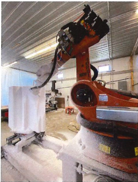
CNC Routed Foam Used for Formwork
