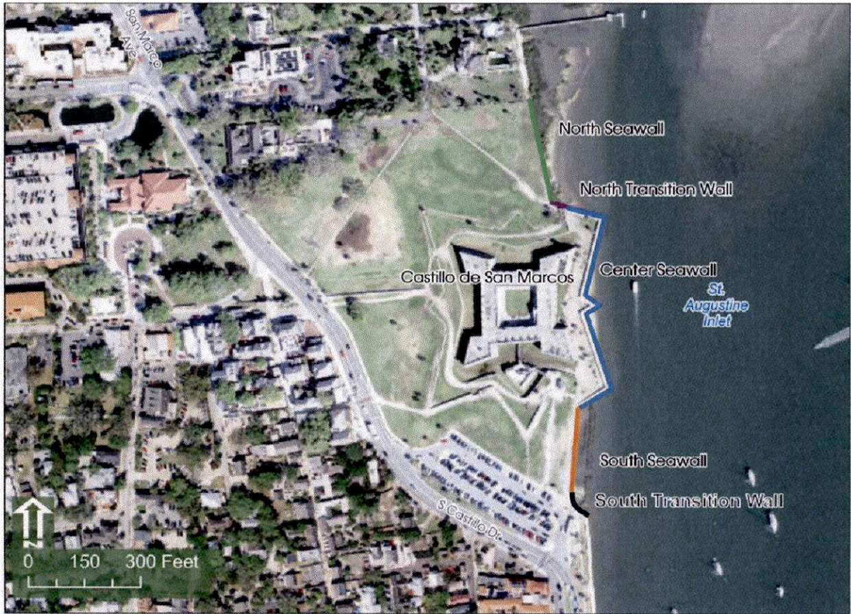
FIGURE 1. FIVE SEAWALL SECTIONS
