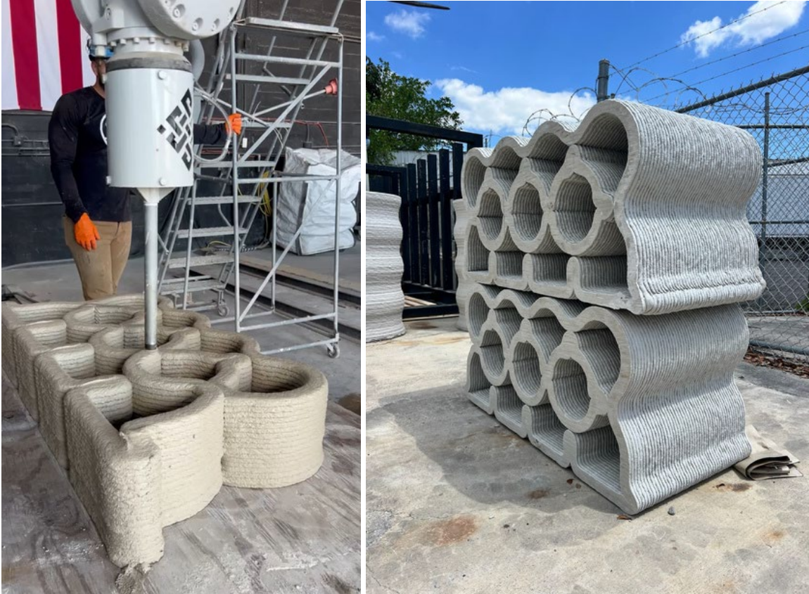
KIND Design’s 3D-Printed Oyster Reef. Photo courtesy of KIND Designs ( www.kindesigns.com ).
