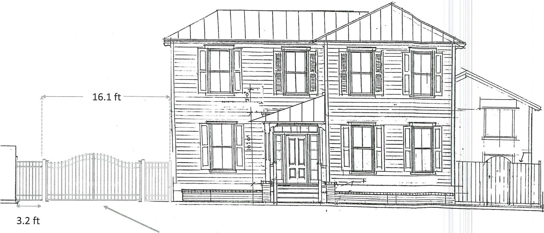
New double swing gate with pedestrian entrance and fence
